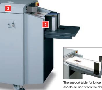
sheets is used when the sheet length is 650 mm / 25.59" or longer. The maximum sheet length which can be loaded is 865 mm / 34.00".
